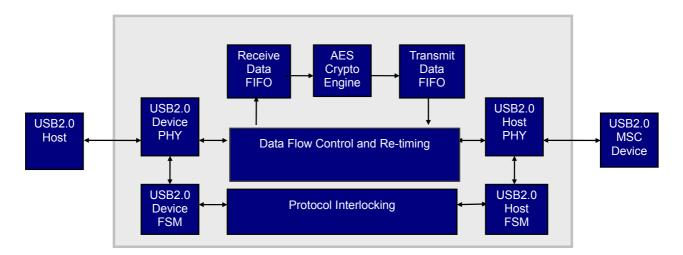
**The** *X-Wall DX USB OTG* sits between the USB2.0/3.0 host and USB2.0/3.0 device, encrypting data before it is written to the storage and decrypting while it is read. The cryptographic operation is totally transparent to users thus produces no performance loss while all data-at-rest are hardware AES 256-bit encrypted. Enova provides customized API library SDK specifically targeting Linux, Windows and Macintosh operating systems.
